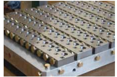
MTS pallet with hydraulic clamping elements.
