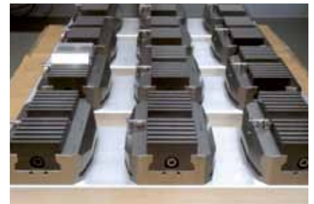
EROWA self-centering vise 148 on MTS pallets.
