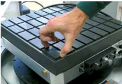
Vacuum clamping on an MTS pallet.
