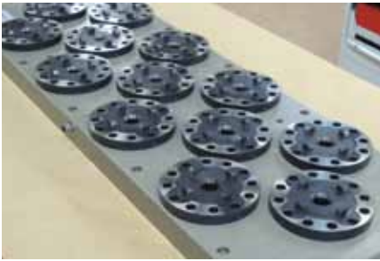
Base plate with 13 MTS single chucks.
