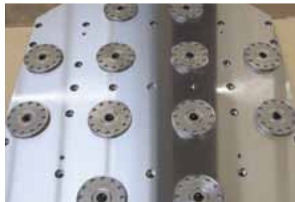
Special MTS base plate, 950 x 950 mm, 12 chucks.
