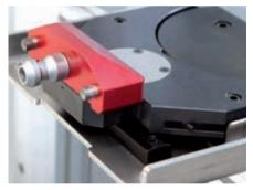
The right gripper for each tooling system size. Stored in the GripperDock and automatically employed when needed.
