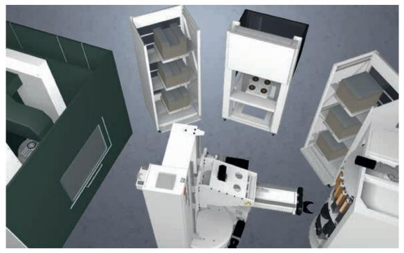
A highly efficient system for automating the manufacture of single parts and small batches. Workpieces are supplied and removed via the integrated set-up and loading stations. When needed, another magazine is added.
