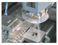
Washing, drying and quality measurement. These important steps are fully integrated in the system. At the end, it puts out completely finished workpieces with a quality certificate!
