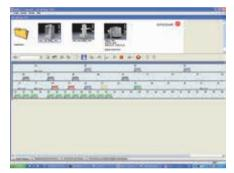
Which tools have to be changed before the end of the day? The display shows exactly how much tool life is left at which position. The system checks internally if the available tool life is sufficient for the released jobs.
