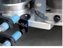
Each magazine position and each pallet is continuously monitored. The EWIS™ Rapid identification system ensures a clear view.
