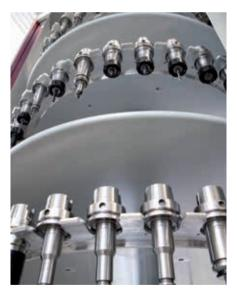
Extending the machine's tool storage; made easy with a Rotary Magazine for tool holders.
