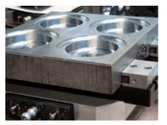
The pallets are equipped depending on the workpiece. Vise, fixture or vacuum clamping plate – EROWA tooling systems get a competent grip on everything.
