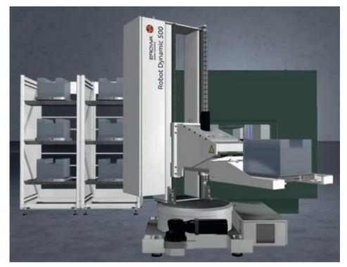
At a first stage, configure the machine such that hours at night can be utilized for the most part. As one magazine is sufficient, at an average machining time of 30 minutes per workpiece, 5 hours can be utilized productively.
