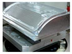
The Robot Dynamic changes pallets with a total weight up to 250 kg reliably on to the machine ...
