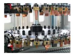
30 positions per level are available for electrode holders. With a maximum of 9 levels, this provides 270 slots.
