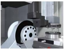
Always the best clamping system size. The robot changes the adapter pallets automatically.
