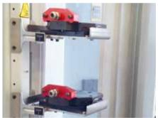
In the gripper dock, various grippers required for the automatic change are stored in a space-saving arrangement.
