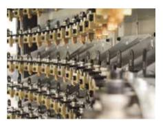
The electrodes are stored in a minimum of space. The Robot Multi has this special magazine.
