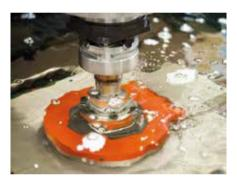
Workpieces and electrodes are loaded automatically onto the EDM machines by the Robot Multi.
