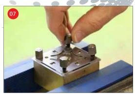
Fit the sealing plate (with new or existing centering plates and supporting feet) to the existing holder.
