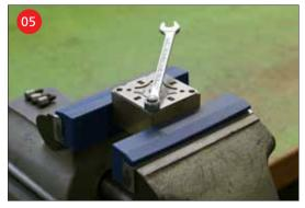
Detach the centering plates from the holders by removing the supporting feet (SW8). Clean the parts that will be put to continued use.
