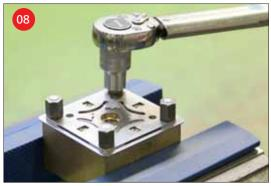
CAUTION: it is imperative that the supporting feet be tightened with a torque wrench (e.g. ER-011600). Torque: 8 Nm.
