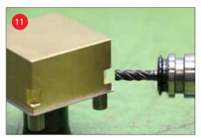
If the retrofitted ITS 50 Holders C are loaded by means of a Robot, then the gripper slot has to be milled.
