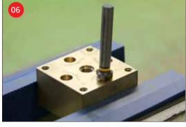
Countersink the  $\emptyset$  8.5 mm boreholes to  $\emptyset$  9 mm x 90°.
