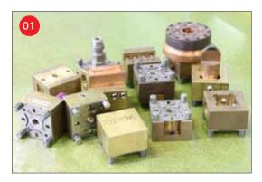
Check the general condition of the electrode holders for damage to the body (thread, contact surfaces for blanks), the supporting feet and the centering plates (worn-out punch holes).
