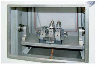
**Cleaning I** The "washing/cleaning" production step is necessary if several processes run in succession automatically. For example, workpiece milling > washing > measuring > EDM.
