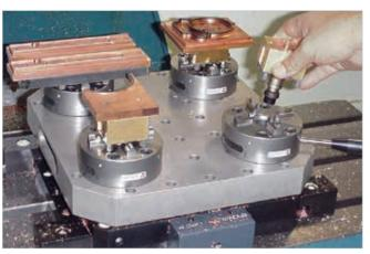
Fixture Manager | Manages several fixtures on a pallet, automatically storing the position of a clamped workpiece. The identification system ensures the correct matching of the data.
