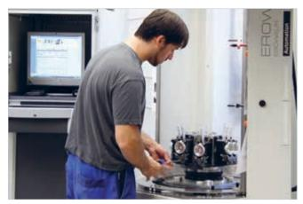
Loading Station | Take the pallet from the tooling station to a free magazine location? The JMS® 4.0 MoldLine does it automatically.
