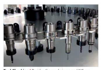
Tool Checking I Besides the workpieces and NC programs, you need the right tools as well. Whether this is the case, and what their remaining lives are, is read from the memory of the machine.
