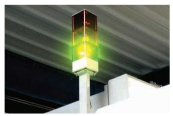
Release I A workpiece is released for machining if all requirements are met. That is, the priority is right, the CNC programs and tools are available, the previous production step has finished, and the intermediate check has confirmed the dimensional accuracy.
