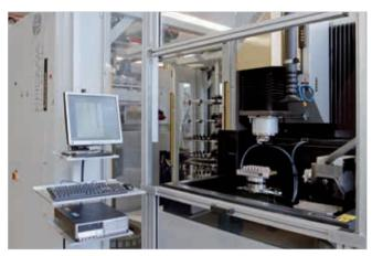
The cell | A production cell consists of the machine, the EROWA robot and the terminal for the process control system. By this, the operator has everything under control.
