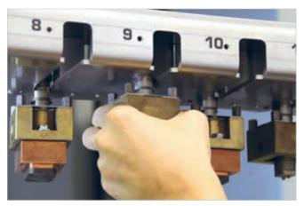
**Job preparation I** Setup and preparation while the production cell is producing. There is no waiting time. The EWIS<sup>TM</sup> chip ensures identification.
