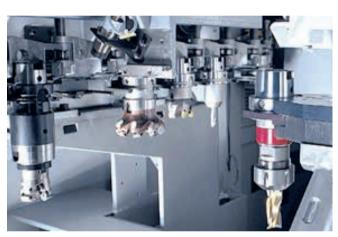
Tool Checking 2 I If a tool is missing or if its life has expired, its sibling tool is used instead. If none is available, the current job is stopped, and the next job on the priority list is processed.
