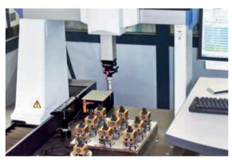
Automatic presetting | The larger the number of produced electrodes, the more important efficient measurement of zero points becomes.
