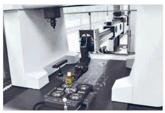
More capacity | Even the "quality measurement" process step can be automated. A potential bottleneck is eliminated by automatic measurements in the second and third shifts.
