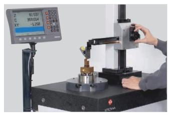
**Presetting I** Offset data of electrodes is determined easily on the PreSet 2D presetting station. The data is associated with the corresponding electrode through the integrated interface.
