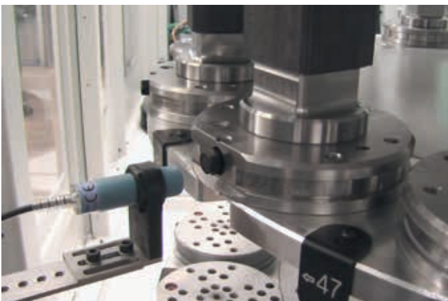
Staged pallets with workpieces are uniquely marked with a chip. At every station in the production process, each pallet is precisely identified by the EROWA EWIST™ system.
