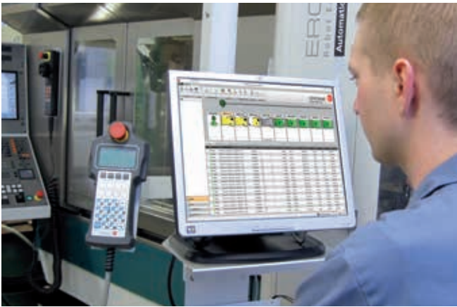
A production cell consists of the machine, the EROWA robot and the terminal for the process control system. So the operator has everything under control.
