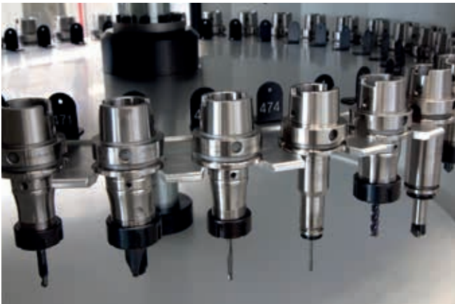
Besides the workpieces and NC programs, you need the right tools as well. Whether this is the case, and what their remaining lives are, is read from the memory of the machine.
